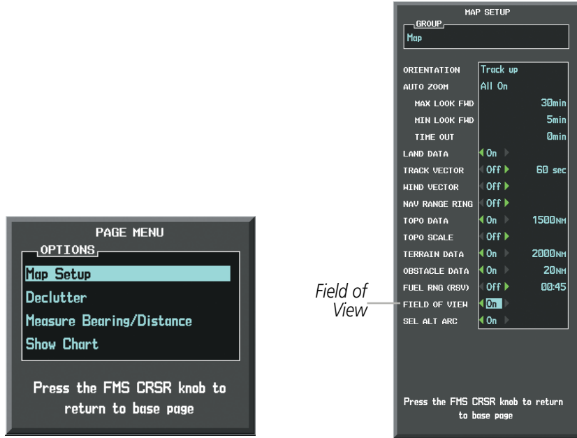
Navigation Map Page OPTIONS Menu Map Setup Menu, Map Group, Field of View Option
